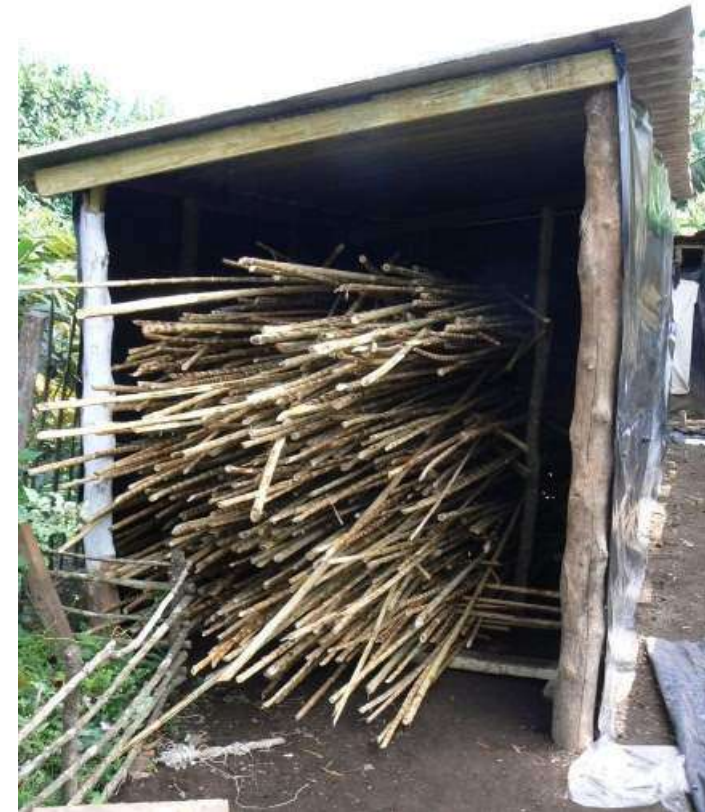
Above: partial seasoning of bamboo left outside but stacked such that air can flow around culms and rainwater drips off
