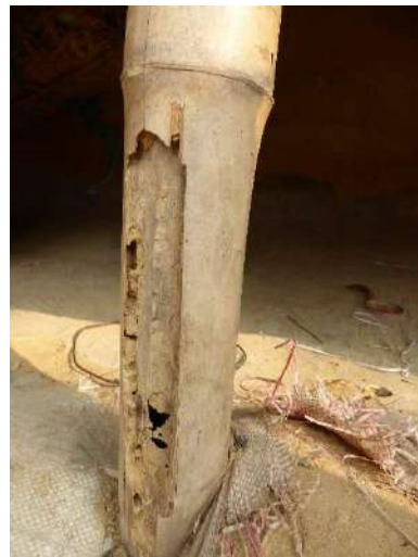
Left: beetle attack in camp; Middle: termite attack in camp
