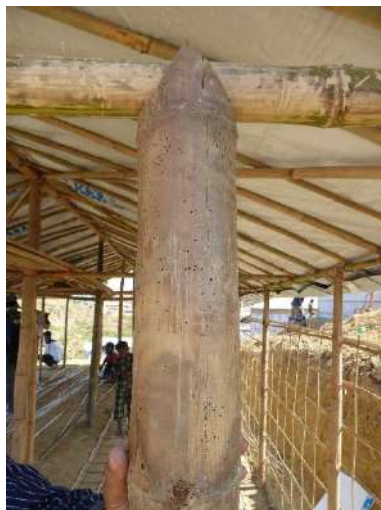
Left: beetle attack in camp; Middle: termite attack in camp
