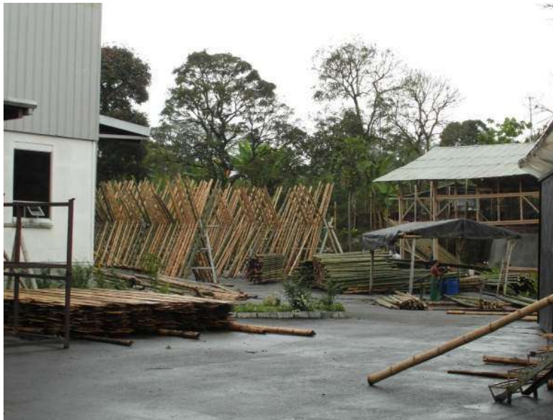
Above: partial seasoning of bamboo left outside but stacked such that air can flow around culms and rainwater drips off
