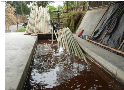
Figure 44: Bamboo treatment bath using boron (Colombia)
