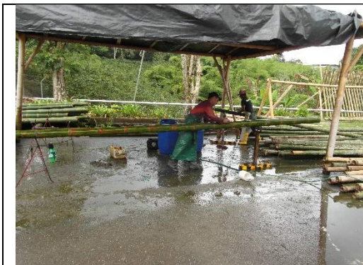
Figure 42: Culms should be cleaned before placing in bath, to avoid adding dirt to bath, which could affect the hydrometer reading (Colombia)
