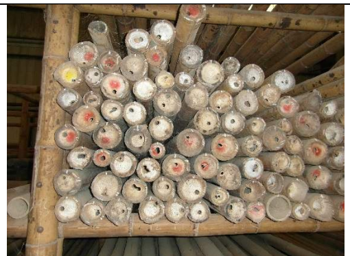
Figure 43: Culms should have their nodal diaphragm pierced as shown, or alternatively each internodal region should have two holes drilled into them (Colombia)
