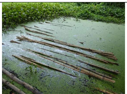
Figure 31: Water treatment of bamboo by immersion in water (India)
