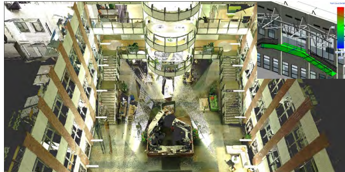
Arup LiDAR scanned the Athenahealth building in Boston to verify construction fitout accuracy.
