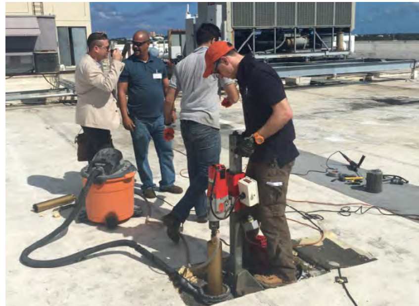
In-situ materials testing of concrete to establish strength and material properties allows appropriate solutions to be developed.
