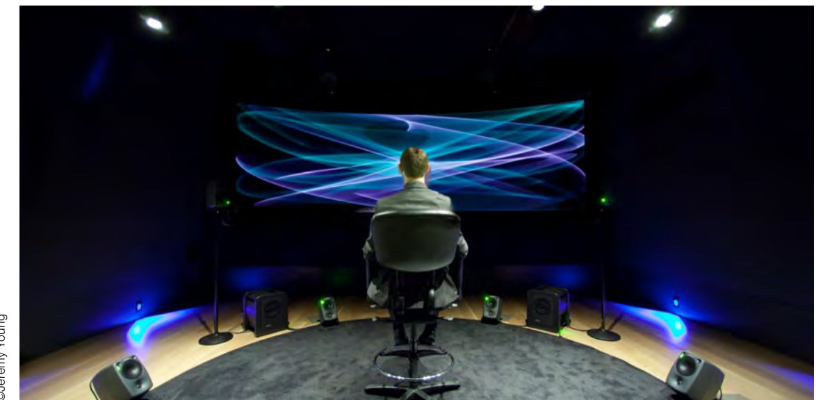
In the Arup SoundLab, we can listen to the acoustics of an existing asset and compare design options for reshaping the sound environment to better accommodate new functions.
