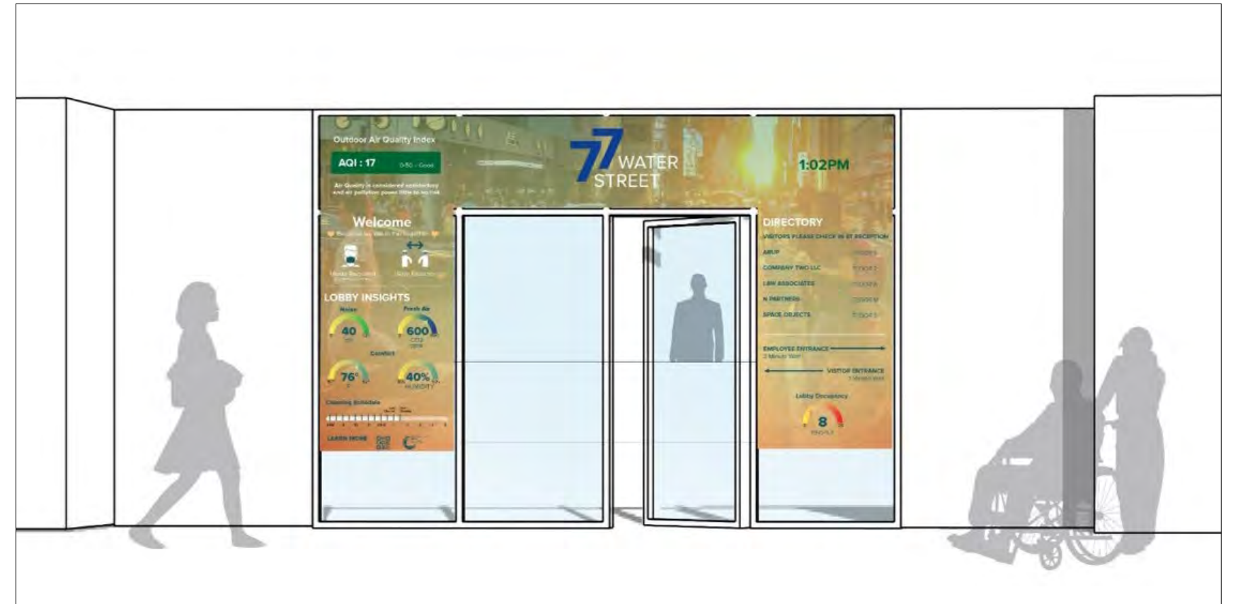
Install a building dashboard at the threshold of commercial office spaces to offer users real-time data on IEQ and health status.
