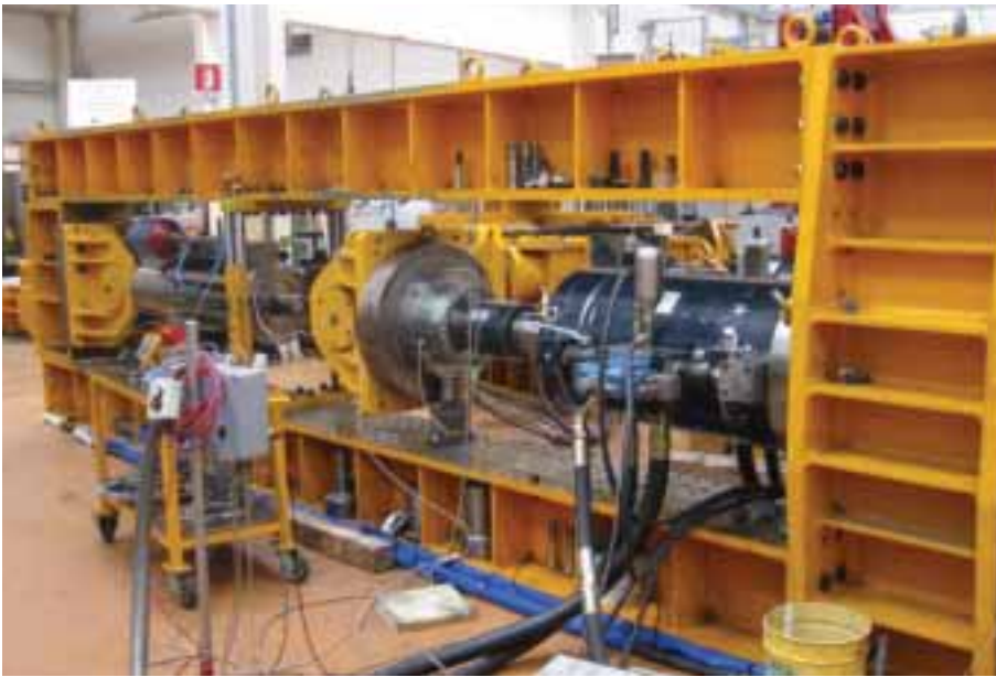
12. Testing the dampers.
