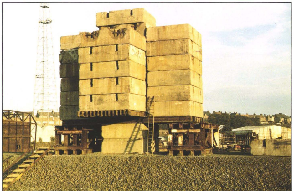
Methil: Sheet pile wall and below: Load test on compacted fill
