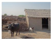
Acceptability – This shelter was weatherproof but with only one opening for the doorway, light and ventilation was limited inside the shelter. No door was provided in the doorway so security was an issue. This shelter was not part of an integrated programme, so space for cooking and WATSAN were not considered.
