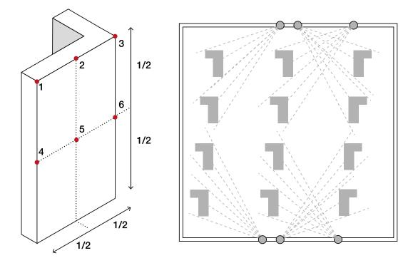
Figure 14 - Total station measurement points on panels, fixed still photos and camera mounts
