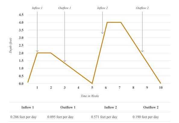
Figure 13 - Flood testing profile - water depth over time and flow rates
