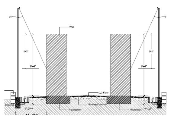
Figure 12 - Section showing two rain test panels with sprinkler and drainage arrangement
