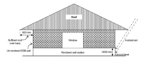
Figure 17 - Hat and boots approach to protecting earth construction (Andabati, D 2010)
