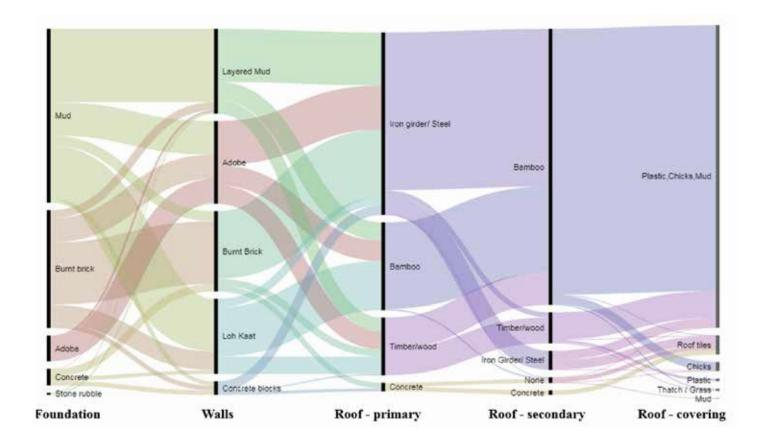
*Figure 15* - Ribbon diagram illustrates which materials were used for foundations, walls and roofing and how often they were used together. For example adobe block foundations were used with adobe walls and a very small number of layered mud walls.
