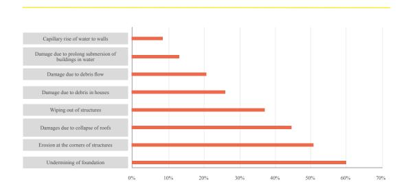
Figure 5 - Major causes of collapse due to mud houses in flood affected areas (UN-HABITAT 2012)
