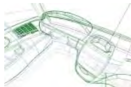
17. Deleting driver's separate door gave larger surface area for switches and controls.
