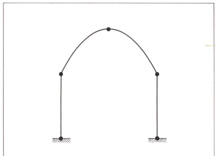
Fig. 1c Collapse of a portal frame
