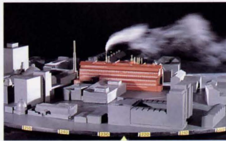
△ 10. Wind tunnel tests for fume dispersal.
