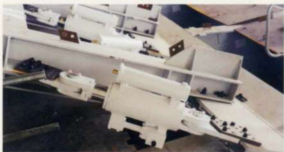
18. Oil cylinder for fuse system.
