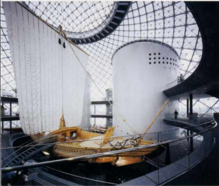
16. The higaki kaisen surrounded by the annular floors. The ship sits on reinforced concrete columns with seismic isolators.
