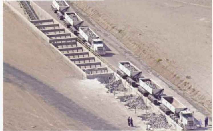
13. Road trains unloading platinum ore at SMC.
