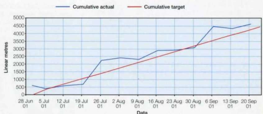
11. Typical line of balance chart for rock fill activity.
