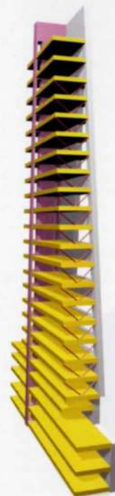
3. The shear walls, core, and façade diagonal bracing form the main structural elements; the structure is pushed to the perimeter to maximize usable floor area.
