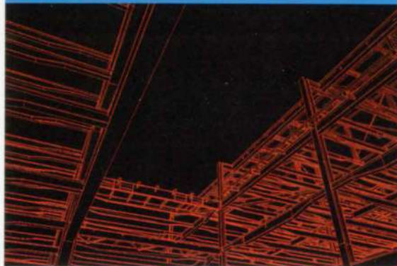
6. Extract from XSTEEL 3D computer model of the atrium structure, without atrium roof details.
