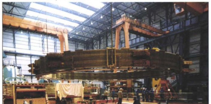
▽ 13. Lower outer poloidal field coil under construction
