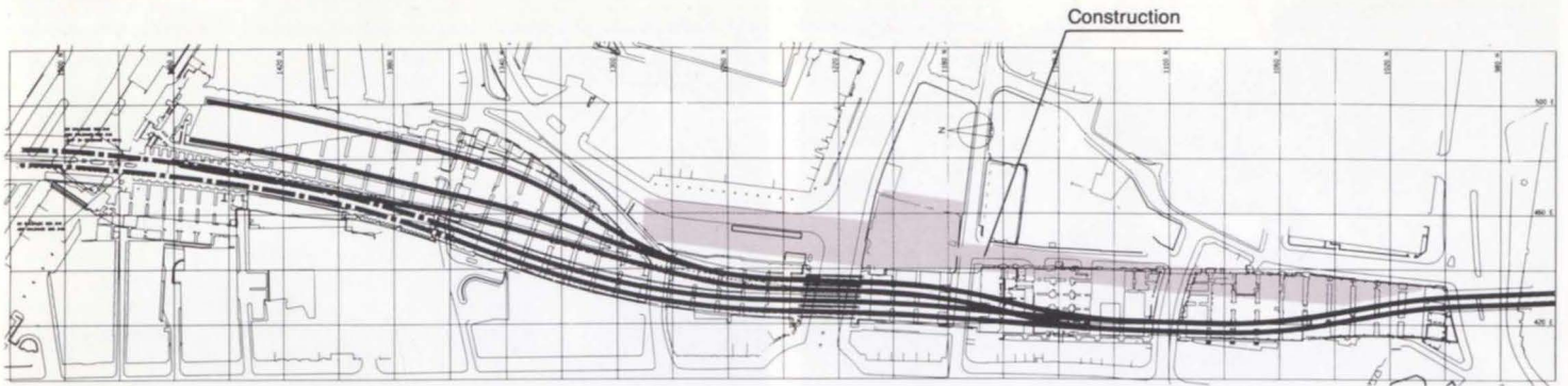
16. Temporary track alignment: Stage 1.
