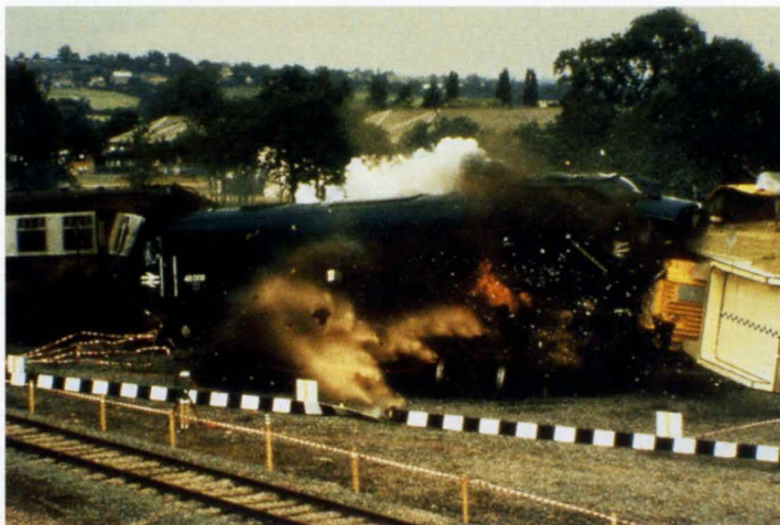
1. Train crash demonstration of the Magnox flask.
