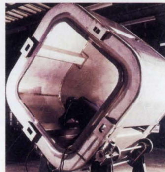
3. The Nirex 3m 3 box during prototype manufacture.
