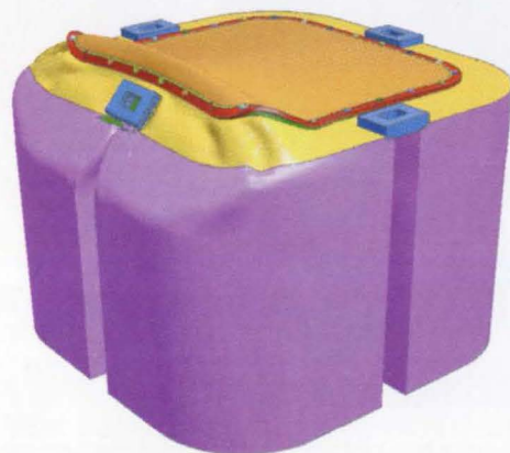
9. Finite element impact analysis of the Nirex 3m 3 box - at the end of a 25m drop.
