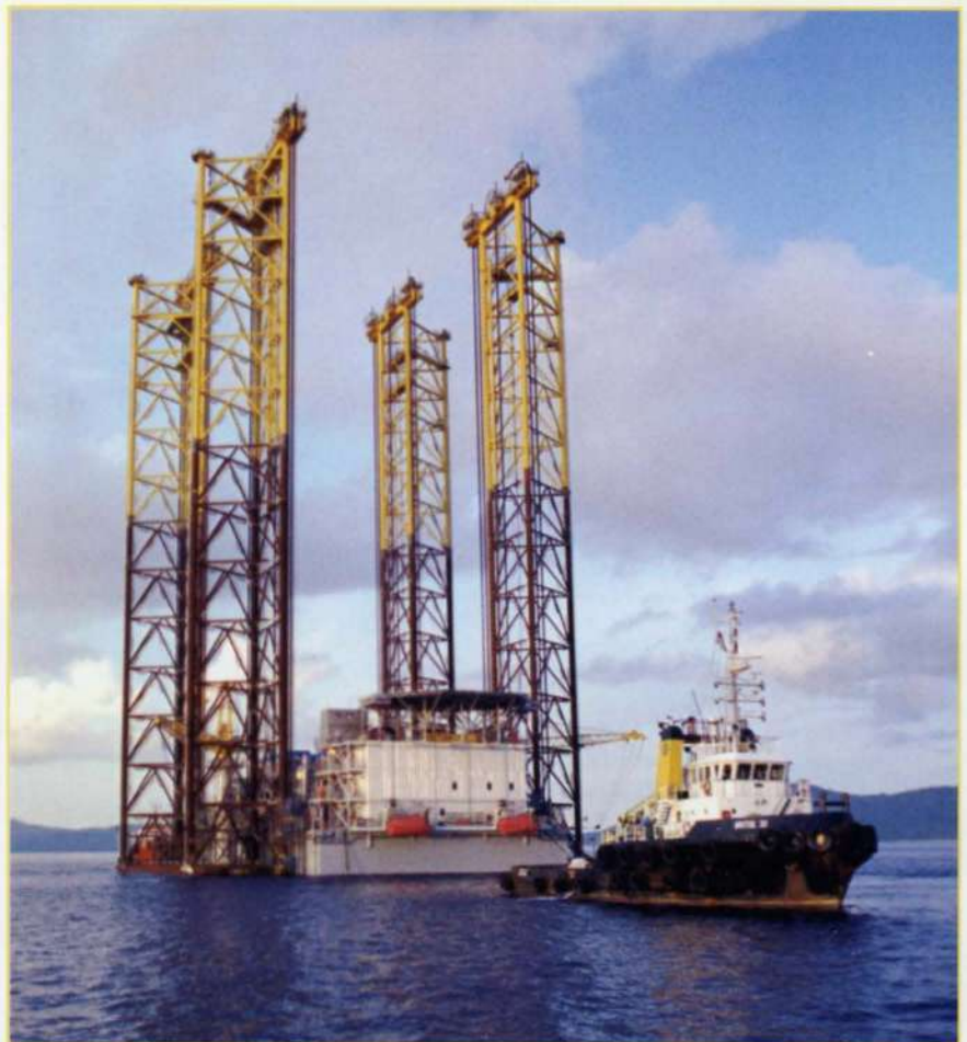
1. Platform ready for wet tow.
