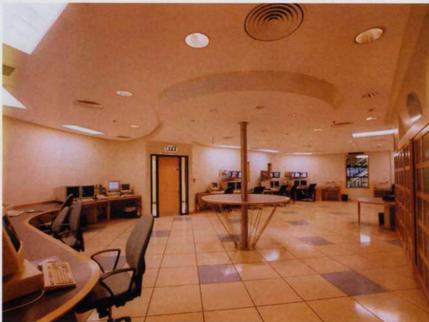
7 left and 8 above. Artificial lighting in the production building control room at different times during the 24-hour cycle. It is manned around the clock, and so the lighting system has been designed to synchronize with the circadian rhythms of the staff.
