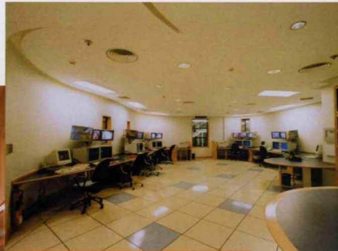
7 left and 8 above. Artificial lighting in the production building control room at different times during the 24-hour cycle. It is manned around the clock, and so the lighting system has been designed to synchronize with the circadian rhythms of the staff.
