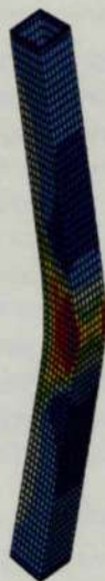
10. Non-linear finite element simulation model showing local buckling of a typical steel brace.
