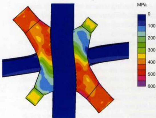
12. The von Mises stress distribution of a large connection plate under the most unfavourable loading combination.
