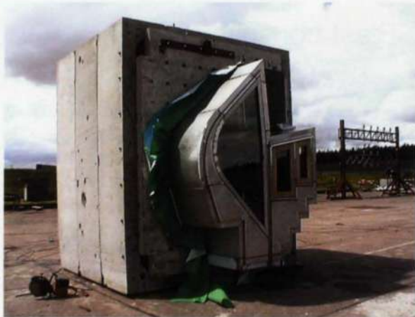
21. Test arrangement for MSP building west elevation window.
