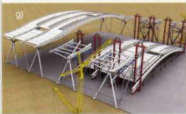
6. Roof assembly sequence.
