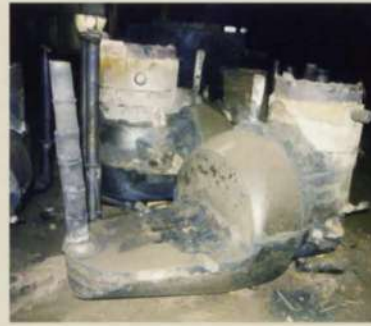
17. Casting removed from sand mould.
