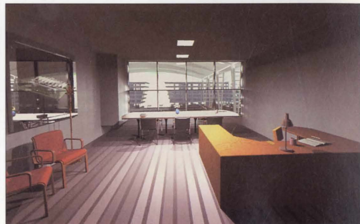
4. Daylight penetration into interior of office, generated by the RADIANCE light visualization program.
