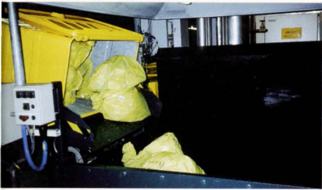
6. Bags of waste being tipped into the incinerator hopper.
