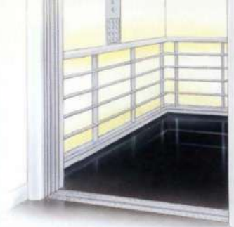
3. Final as-built design concept for interior, with 'bull bar' protection for lower level glass.
