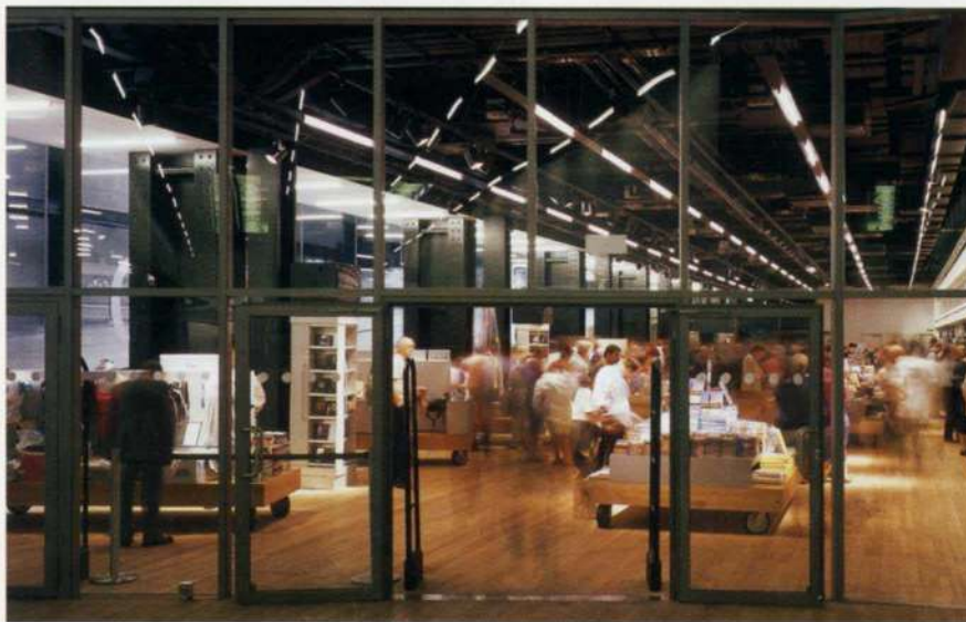
2. Exhaust air from the galleries is used to moderate the Turbine Hall environment. Glazed bay window enclosures provide lighting to the Turbine Hall.
