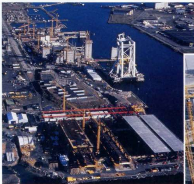
3. Pier shafts were cast at the Malmö yard.
