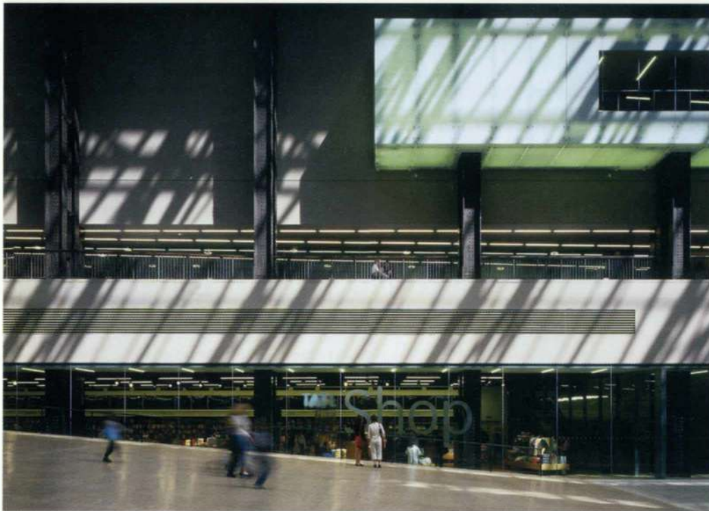
2. Exhaust air from the galleries is used to moderate the Turbine Hall environment. Glazed bay window enclosures provide lighting to the Turbine Hall.
