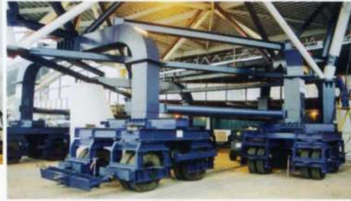
6. Blue-painted steel temporary carrying chassis beneath node.
