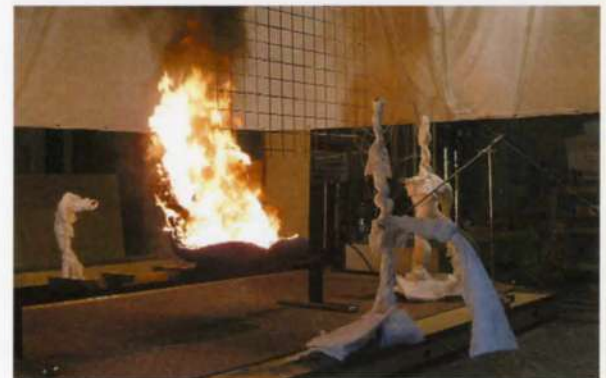
17. Combustion test on fire resistance of steel elements.
