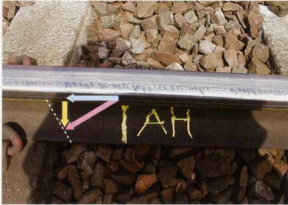
9. Surface crack angle as a function of contact patch longitudinal and lateral forces.
