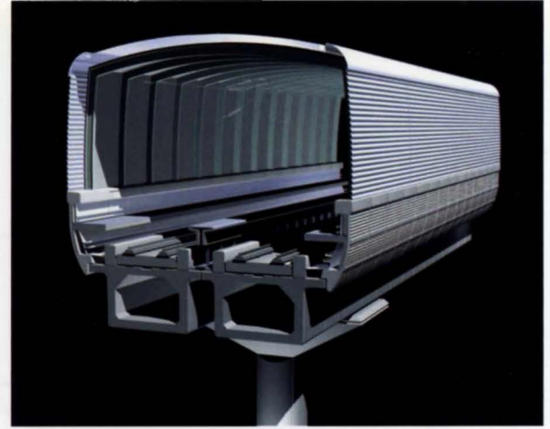
12. Design for full noise enclosure at crossings.
