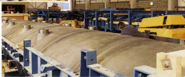
9. Steel moulds for floor units.
