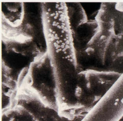
8. Self-healing materials: hollow fibres filled with active chemicals.
