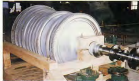
7. Turbine assembly on site in the Energy Centre.
