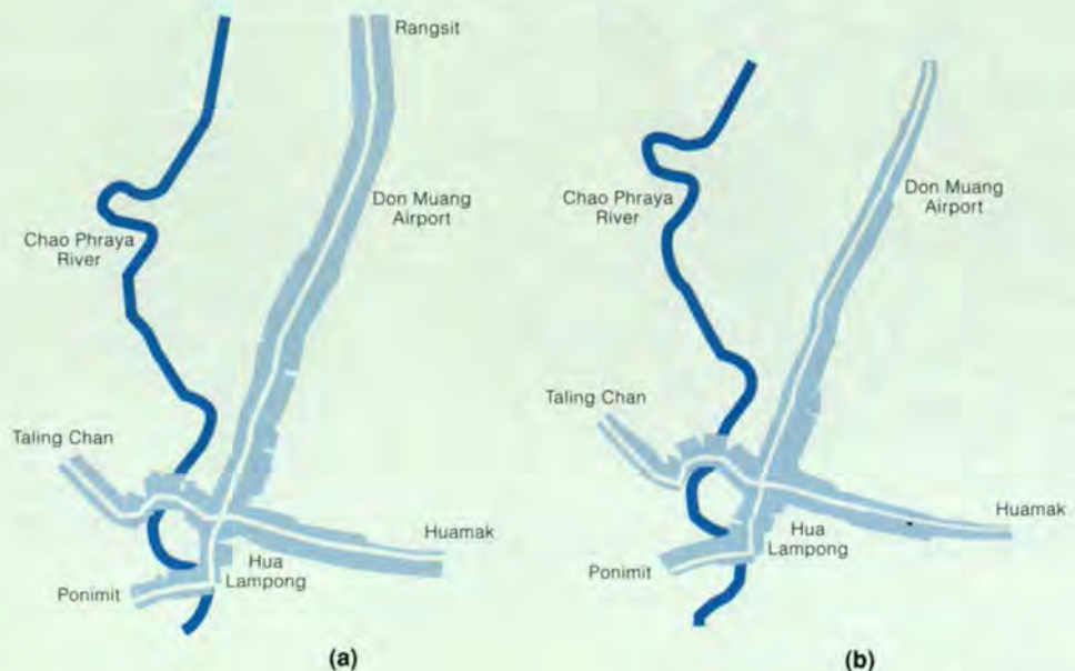
5. Forecast demands for BERTS; (a) tollway (bandwidth indicates scheme loading in am peak period); (b) CT system (bandwidth indicates scheme patronage in am peak period).
