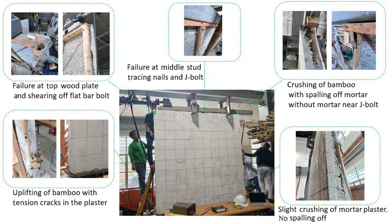
Figure A8.5: Typical damage mechanisms seen in CBSW panels
