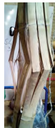
Figure 6.5: Axial failure of G. Angustifolia culm 6.5
