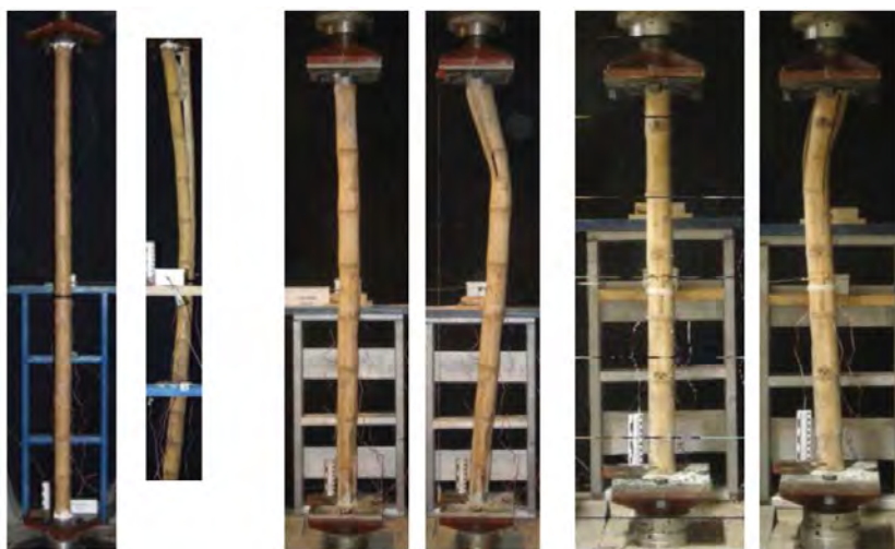
Figure 6.4: Single B. stenostachya culms subject to axial load 6.4
